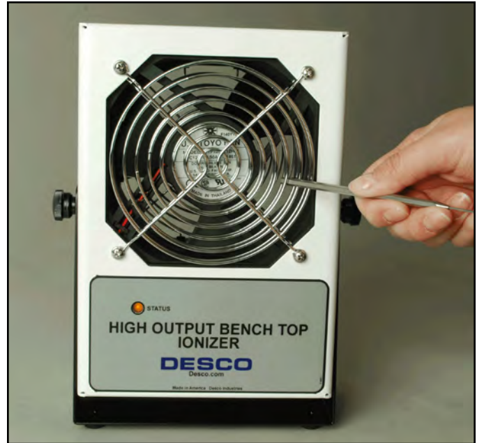
Figure 7. Shorting the ionizer's fan grills with a metal probe to test the alarm
